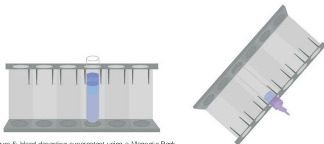
Figure 5: Hand-decanting supernatant using a Magnetic Rack.
