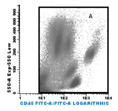
Acquire and analyze sample in the tube as much as possible. It is recommended to acquire at low or medium speed to avoid the formation of cell aggregates. If you will not acquire the entire sample is advisable to stop every 4 minutes, shake the tube manually and proceed with the acquisition.
